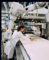
Research at the online pre-preg system, which is used at CZM to produce high-performance components from fiber composites.
